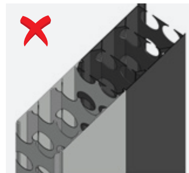
Incorrect – web holes do not align
